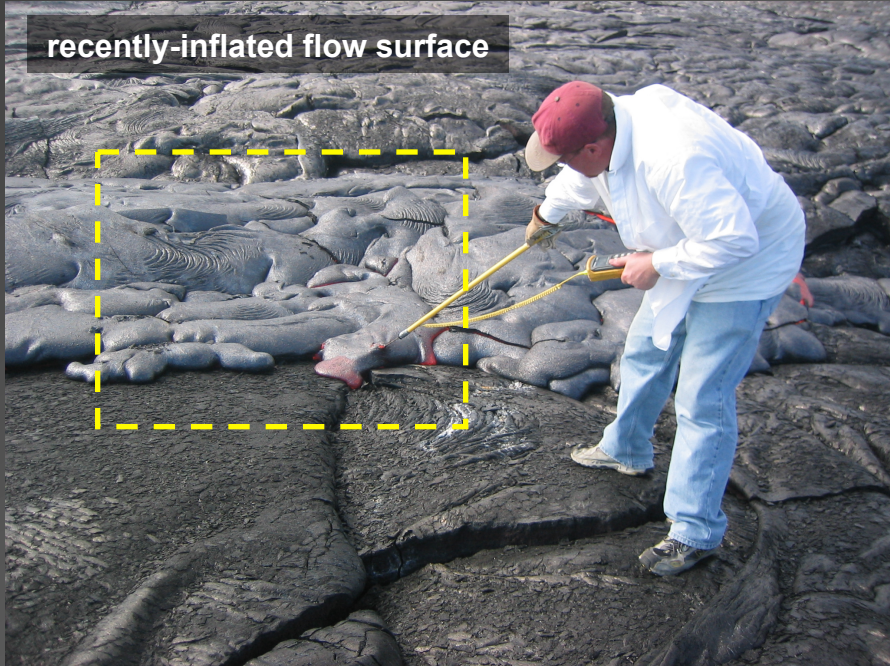
digital video image capture showing thermocouple measurement
