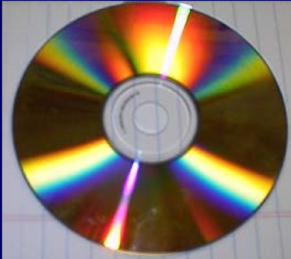
Interferometric fringes on a CD
