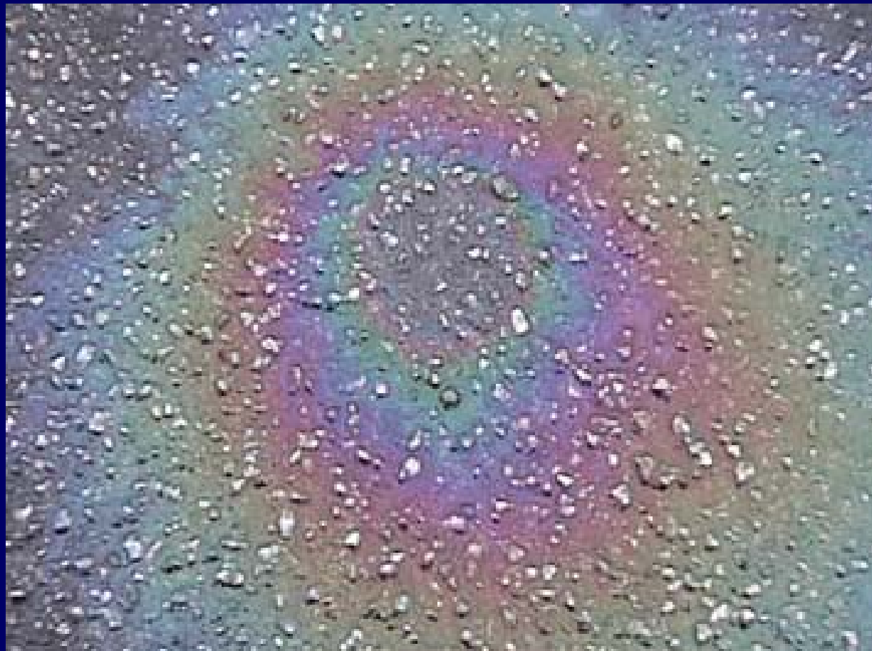
Interferometric fringes on an oil film
