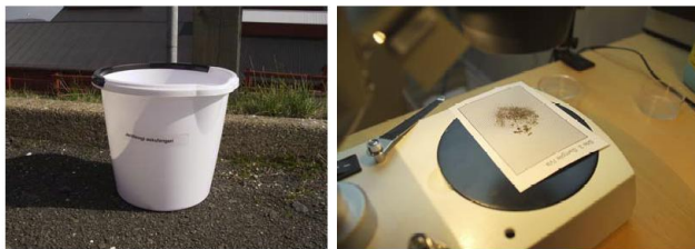
Fig 1. Views of the sample container positioned in the car park of the Faroese Earth and Energy Directorate in Hoyvik, Streymoy, Faroe Islands and the first sample collected from the Eyjafjallajökull eruption. This sample weighs ~50 mg.
