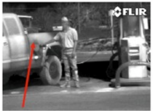
Figure 2B. Gasoline vapors wafting from the nozzle of a non-vapor recovery hose.
