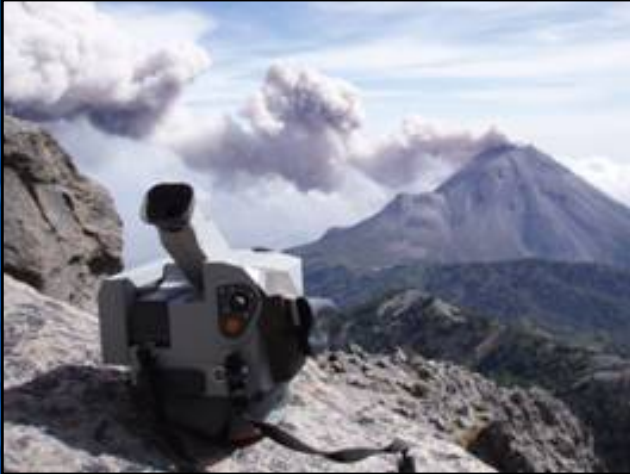
VarioCAM infrared camera 8 – 13.5 \mu\text{m}
