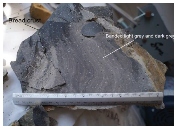
Fig. 4 – Fragment of bread-crust bomb with outer dark glassy rind and distinct interior displaying parallel flow-banding. Layers of micro-vesicular light-grey material alternate with denser dark-grey layers. Larger xenolithic enclaves (< 2 cm) surrounded by bands are common. All layers contain micro-phenocrysts of Plag (~2 mm), Ol (~1.5 mm), and biotite (~1 mm). The crust is richer in Plag than the core, but the core is richer in biotite.
