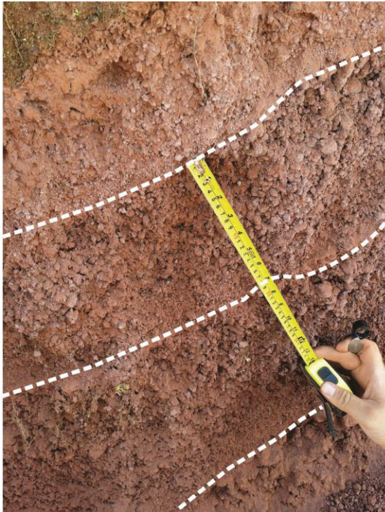
Fig. 4 – Lapilli and ash deposit with reversed graded bedding exposed in Los Chiles hill.
