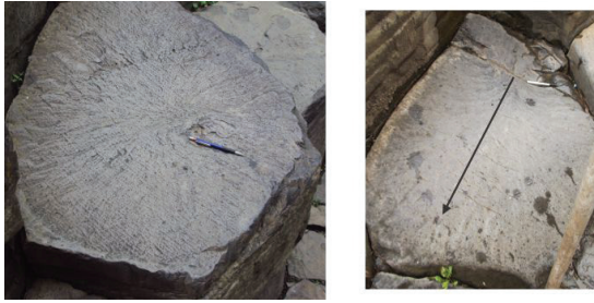
Figure 3. Radiating striae (left) and plume-like striae with a symmetric line (right). The arrow indicates propagation direction of the fracture.
