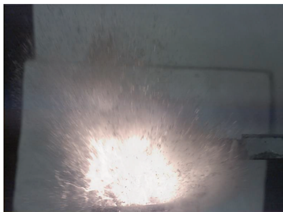
Fig. 2 – Early part of post explosive expansion phase. High velocity cool particles separate from low velocity hot particles. Melt from basaltic eruption of Grimsvötn 2004 (Iceland) at 1200 °C. Frame from high-speed recording at 5000 fps, aperture time 100 µs, size=65 x 50 cm.
