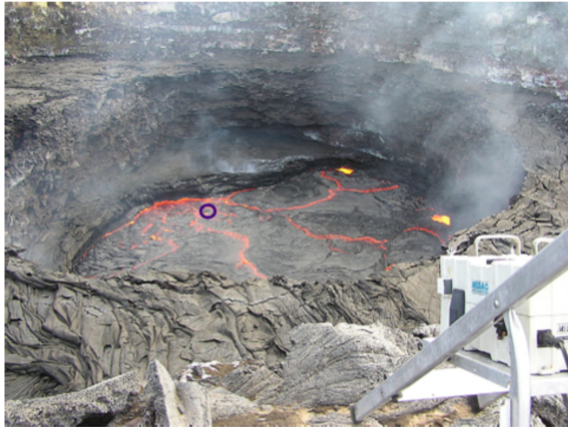
Fig. 2. Photograph of Erta 'Ale lava lake from the observation site on the north eastern rim of the central pit. The black circle approximates the 1.5 m 'footprint' of the FTIR spectrometer.
