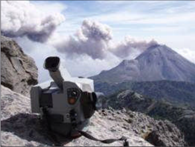
VarioCAM infrared camera 8 – 13.5 \mu\text{m}
