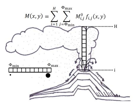
For each step up the eruption column (i), from the vent to the maximum column height, each grain size (j) is considered. Tephra2 calculates the probability of particle release at each step. Once a particle is released, the particle fall time is calculated based on the point of release.
