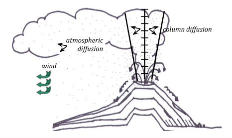
Particle movement is modified by both column diffusion and atmospheric diffusion. Particles fall through a layered atmosphere, with layers characterized by different wind velocities. In this manner, mass is accumulated at each grid location.
