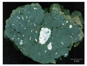
Fig. 2 – Composite, domainal clast of basalt containing unmelted rhyolite fragments. Rotomahana maar deposits, New Zealand. (See Rosseel et al., 2006)
