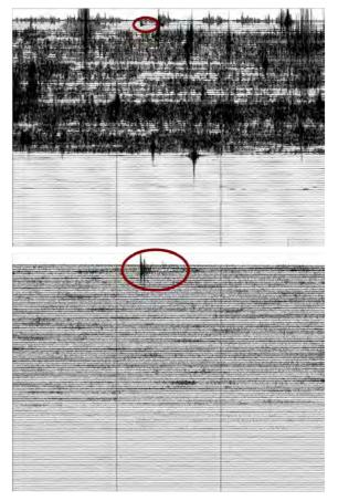
Fig. 1 - Helicorder plots recorded at Riverhead (north Auckland, see map Fig. 3) starting in the morning and going into the night of 11 April 2007. Seismograms are from the surface seismometer (*Top*) and the borehole seismometer at 245 m depth (*Bottom*). Time along the x axis is 3 minutes. The plots are not shown on the same scale due to the high amplitude of the noise. From Ashenden et al. (2011).
