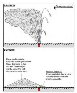
Fig. 3 – Schematic sketch showing the effect of strong cross-winds on an eruption plume and ballistic ejecta, as well as the main characteristics of the resulting deposits.
