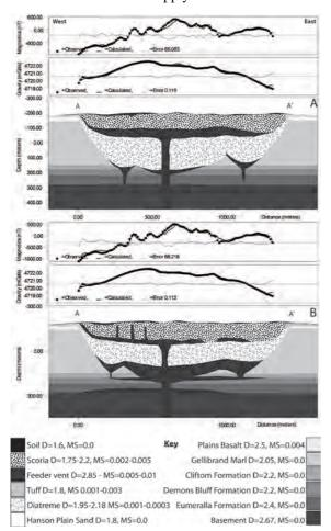
Fig. 1 - 2D forward models across the MNVC, constructed to correspond to east – west magnetic and gravity transects (transect A – A'). Model A displays ponding of rewelded spatter in the crater of the coalesced maars. Model B displays intrusion and inflation of magma along the base of the diatremes.
