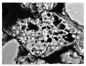
Fig. 1 - Back scattered image of a fine ash particles in a polished thin section of wet phreatomagmatic pyroclastic ash. The clast in the middle has a relatively high vesicularity in contrast to the surrounding dense clast.
