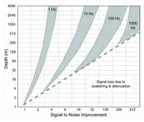
Fig. 2 - Expected improvement of signal to noise ratio with increased seismometer depth. Based on empirical data, Peter Malin and Ashenden et al. (2011).
