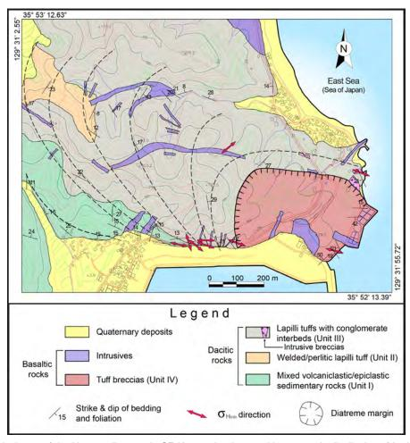
Fig. 1 - Geological map of the Yangpo diatreme in SE Korea, showing roughly concentric distribution of bedding traces and approximately radial alignment of mafic dikes with respect to the diatreme. The directions of horizontal minimum stresses are generally normal to the strikes of adjacent dikes, suggesting contemporaneous formation of faults and dikes.
