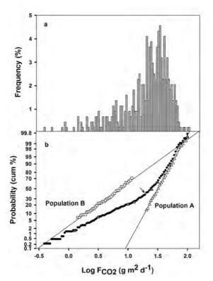
Fig. 1 – Soil gas  $CO_2$  fluxes measured in November 2010 in the Auckland Volcanic Field, as described by a geographical statistical approach. Histogram (a) and probability plot (b) of  $CO_2$  flux data (black circles). Populations A (open triangles up) and B (open squares) are shown as straight lines. The inflection point is indicated by an arrow and corresponds to 67% of population A and 33% of population B.
