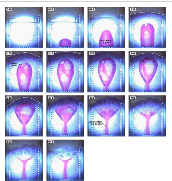
Fig. 2 – A sequence of grabbed video frames from a laboratory-scale cratering experiment run conducted showing an erupting run, akin to those inferred to have occurred at Rotomahana during the 1886 event, (Ross and White, 2006). After Ross et al. (2008).
