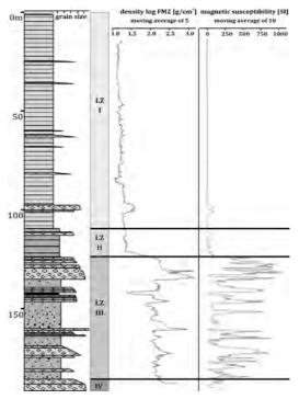
Fig. 1 – Lithology, density log and magnetic susceptibility of post-eruptive central crater sediments at Foulden Maar
