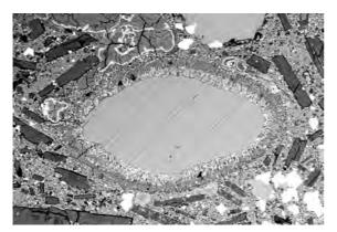
Fig. 3 – Backscattered SEM image showing a reaction rim around a phlogopite crystal. Dark, lath-shaped melilite crystals stand out from a finer matrix. Width of image is 540  $\mu m.$
