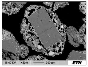
Fig. 3 – Backscattered image of a lapillus from the 2007-2008 eruption of Oldoinyo Lengai. Nepheline crystal cored with melt. Note the high abundance of vesicles in the melt.
