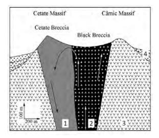
Fig. 1 - Simplified model of the Cetate phreatomagmatic breccia pipe genesis with non-axial position of the fluidization channel (Black Breccia), respectively the set up of a fluidization cell (from Tămaş, 2002). Legend: 1 – Cetate Breccia (sensu stricto, Leary et al., 2004); 2 – Black Breccia; 3 – Cetate dacite; 4 – vent breccia; arrows – transport direction within Cetate Breccia (sensu lato, Tămaş, 2002).
