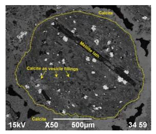
Fig. 2 – Backscattered SEM image of a spherical pyroclast from Mianmoja Hill. Note the large melilite lath near the centre and the infilling of secondary calcite in vesicles.
