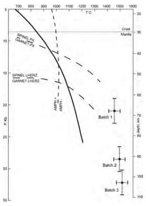
Fig. 3 – Southeast Australian geotherm (O'Reilly and Griffin, 1985) showing the estimated temperatures and depths of origin of the most primitive magmas of Mt. Rouse.
